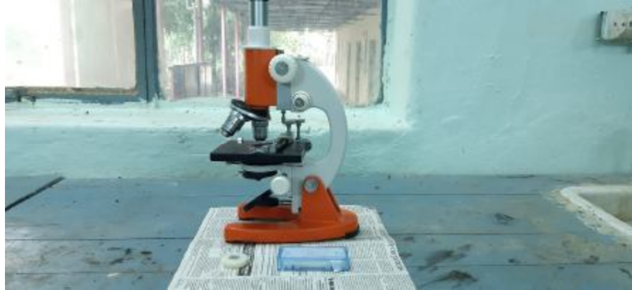
Monocular Microscope with stage and ocular micrometer used in measurement of mycorrhiza spore
